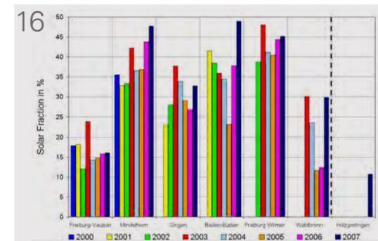
The solar thermal system in the student residence Freiburg-Vauban lies outside the normal range because of the relatively high hot water consumption. Freiburg-Vauban is different due to the high hot water consumption compared to the small collector area. The solar fraction in Holzgerlingen is much lower as the roof area is limited and cannot be enlarged.
