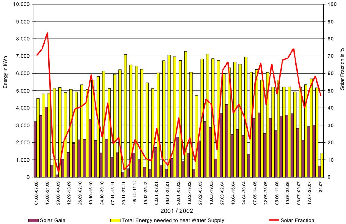
Fig. 4: Solar fraction, solar gain and total energy needed for potable water heating and solar gain in the monitored period from 01.08.2001 – 31.07.2003 in the solar plant in Baden-Baden
