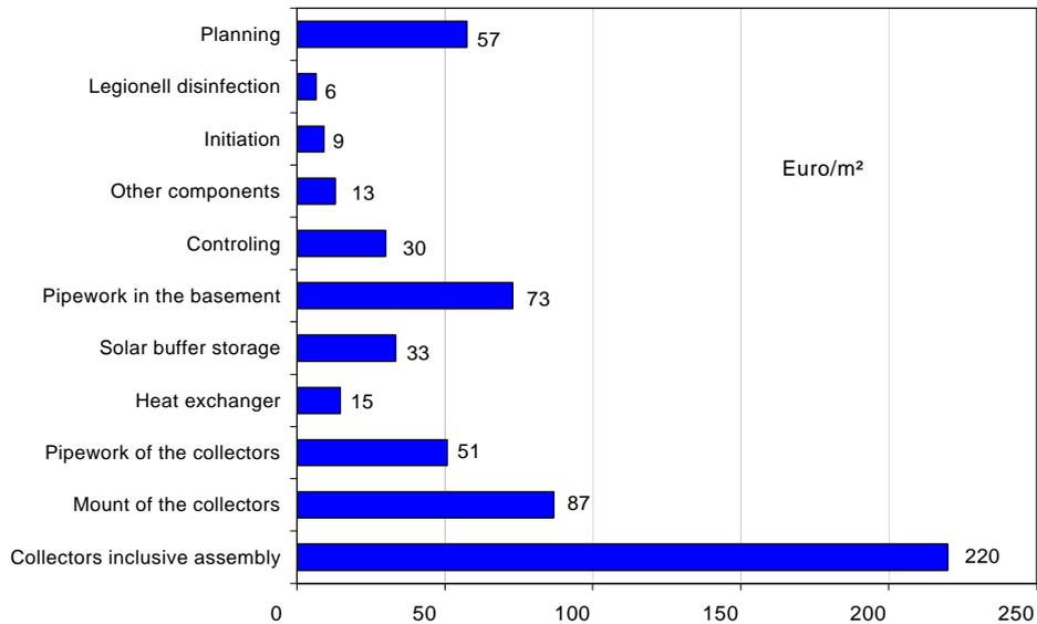
Fig. 3: Solar system costs fractionated on the components
