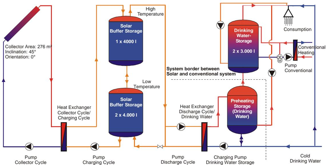
Fig. 2: Hydraulic Scheme of the solar thermal plant in Baden-Baden
