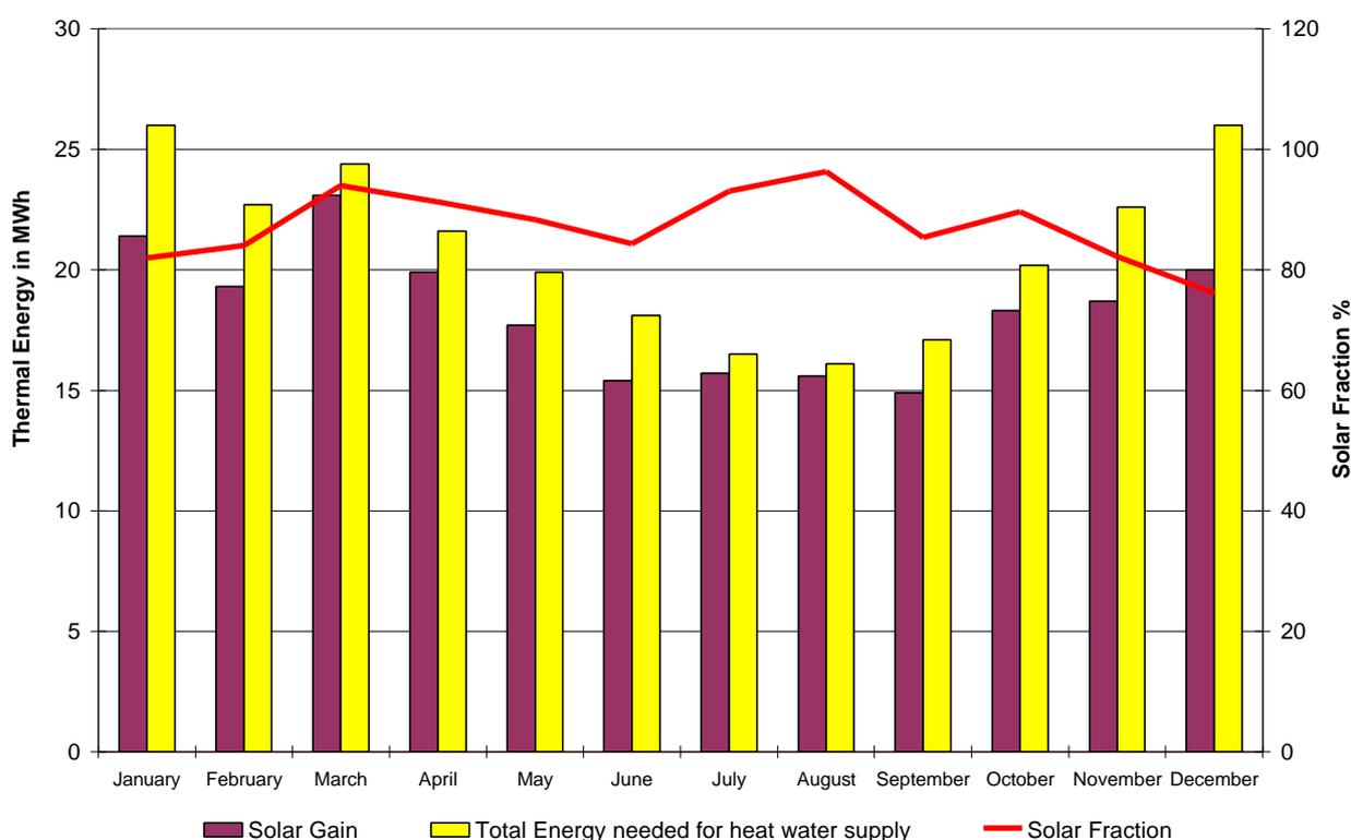
Fig. 6: The solar system of Baden-Baden simulated with the weather data of Camaguey in Cuba
