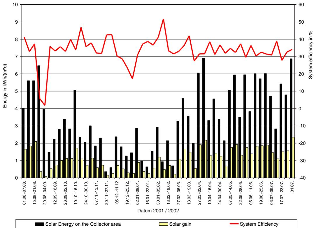
Fig. 5: Solar gain and system efficiency in the first monitoring period 01.08.2001 - 31.07.2002 in the solar plant in Baden-Baden
